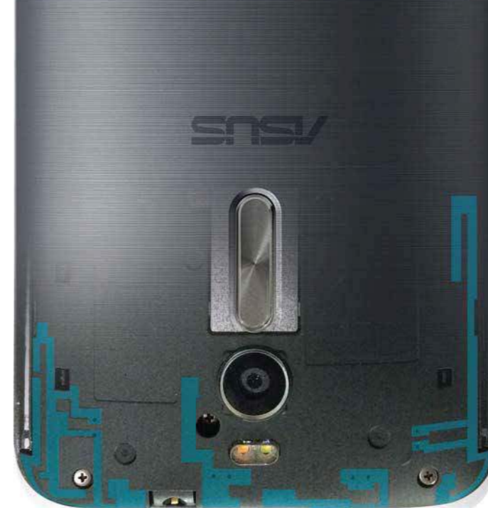
SIM 1 Diversity Antenna 802.11ac Wi-Fi Bluetooth 4.0 5 Satellite GPS SIM 2 Antenna
