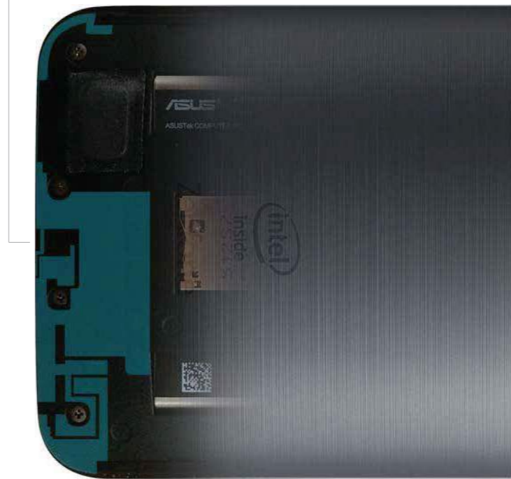
SIM 1 - Main Antenna (2G / 3G / 4G)
