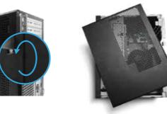
Step Turn the screw to release to lock Step Z Remove the side and front cover
