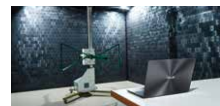
EMI Test This ensures that ASUS laptops perform well in internal or external electromagnetic fields.
