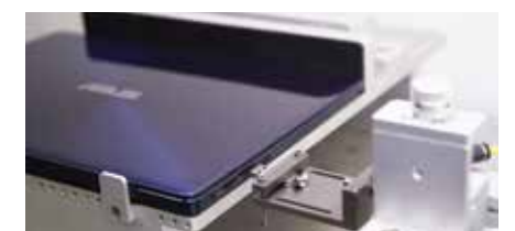
Port Test Port tests ensure that contacts and plugs are durable even in environments where devices are frequently connected and disconnected.
