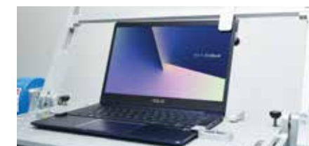
Enhanced Hinge Test Vigorous testing with over 20,000 open/close cycles helps ensure exceptional hinge strength.
