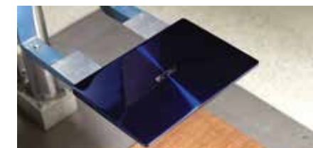
Drop Test Drop tests check the resistance of the chassis and internal components to damage from unexpected drops.
