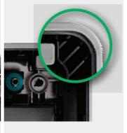
Each corner has reinforced structures which absorb hard impacts.
